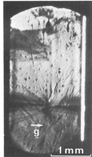
Figure 5 X-ray topograph of a \text{TmAsO}_4 plate recovered from the body of a solidified melt. Note the non-crystallographically oriented defects, the good anomalous transmission, and the few surface defects. ( \text{MoK}\alpha_1 radiation, 200 reflection).
