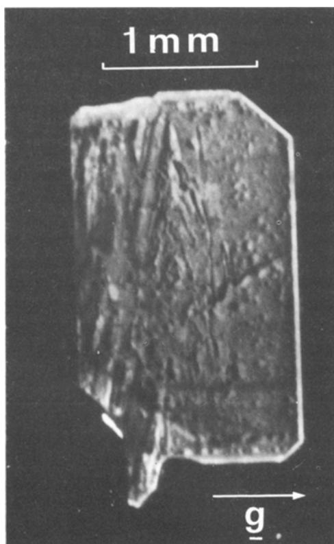
Figure 8 X-ray topograph of a \text{Lu}_{0.98}\text{Tm}_{0.02}\text{AsO}_4 crystal grown in a welded crucible. ( \text{AgK}\alpha_1 radiation, 200 reflection).
